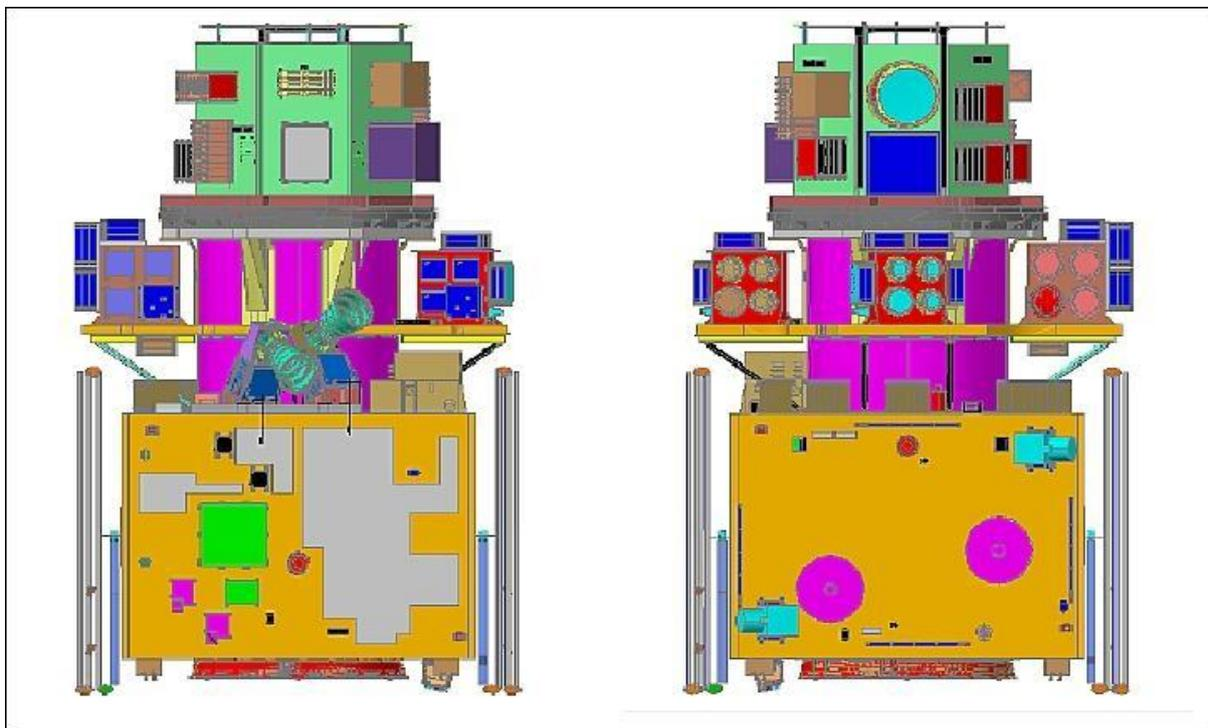
**Figure 2: ResourceSat-2 spacecraft as view from -yaw (left) and as viewed from +yaw (right), image credit: ISRO**
