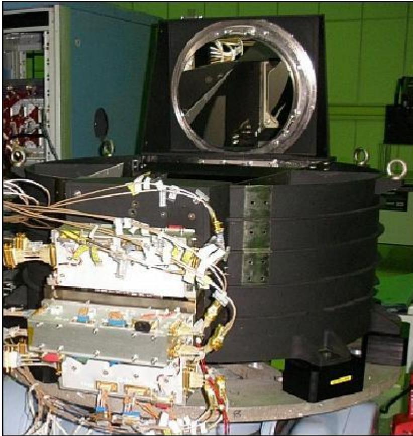
**Figure 16: Photo of the LISS-4 camera (image credit: ISRO)**
