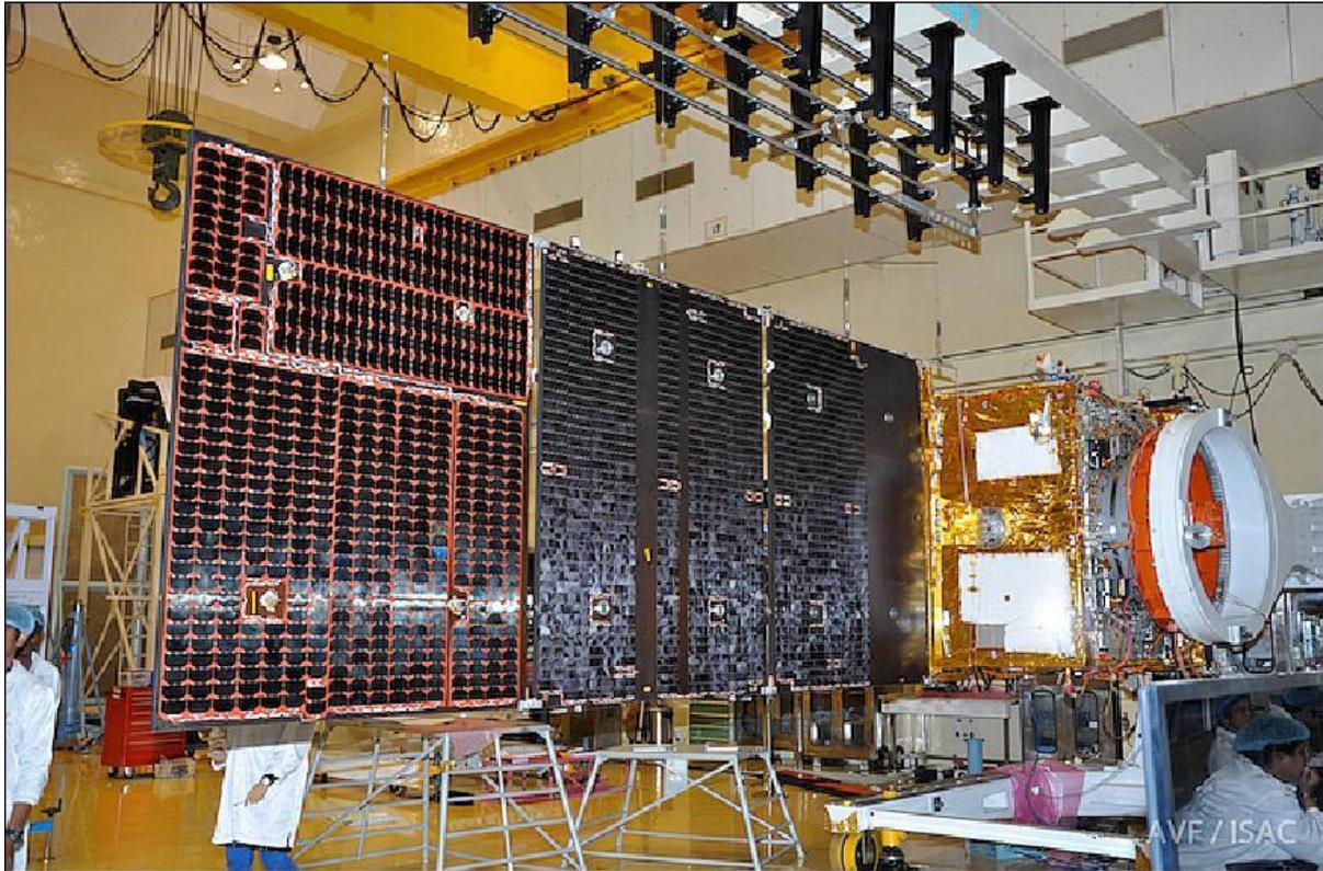
**Figure 5: Photo of the ResourceSat-2A spacecraft at ISRO with deployed solar panels (image credit: ISRO)**
