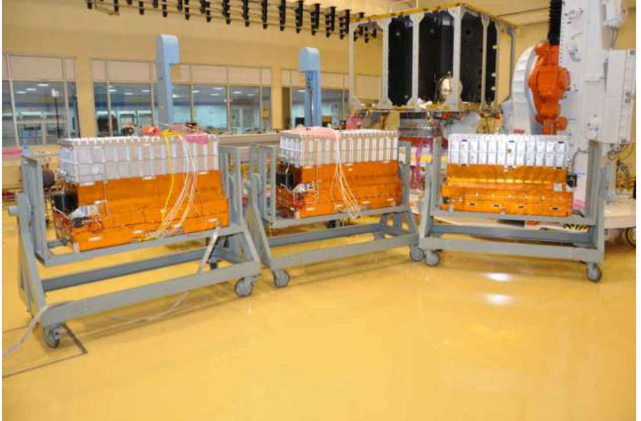
All the three LAXPC flight detectors in Assembly, Integration and Testing lab (AIT) lab of ISAC after successfully completing all flight tests and final calibration (20 th October, 2014). The purification pump is seen as black box in each detector. At the top is the protection cover which was removed before the launch
