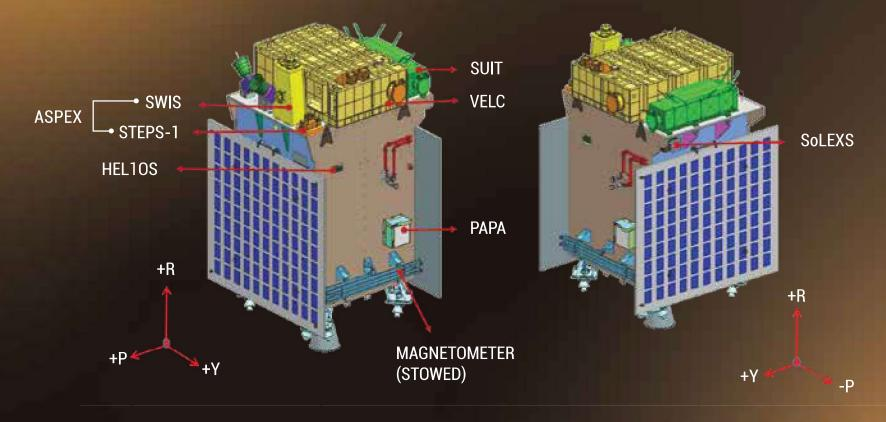
R, P, and Y indicate the Raw, Pitch, and Roll axis of the spacecraft.
