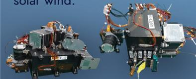
Suprathermal and Energetic Particle Spectrometer is a high-energy spectrometer designed to measure high-energy ions of the solar wind.
